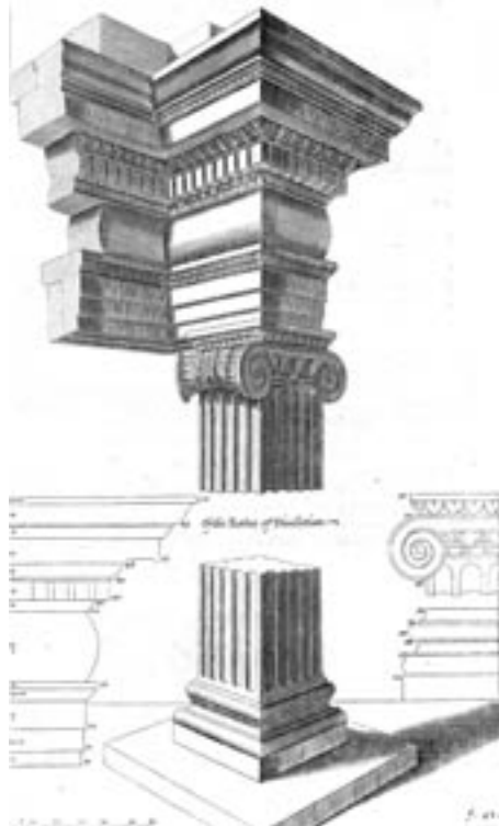
An Ionic entablature from the Baths of Diocletian. The 'rafters' are supported on a 'pulvinate frieze' The 'frieze, (Italian 'fregio'), was a term invented by the Italian Renaissance. The Greek terms were 'zone', as in 'horizon' and 'zoophoros', meaning 'life-bearing'.
