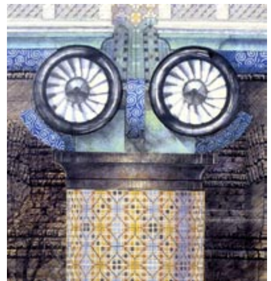
The cylindrical beam-ends to the Entablature on the Blackfriars columns doubled as ventilation fans, after the model of our Isle of Dogs Pumping Stn.
