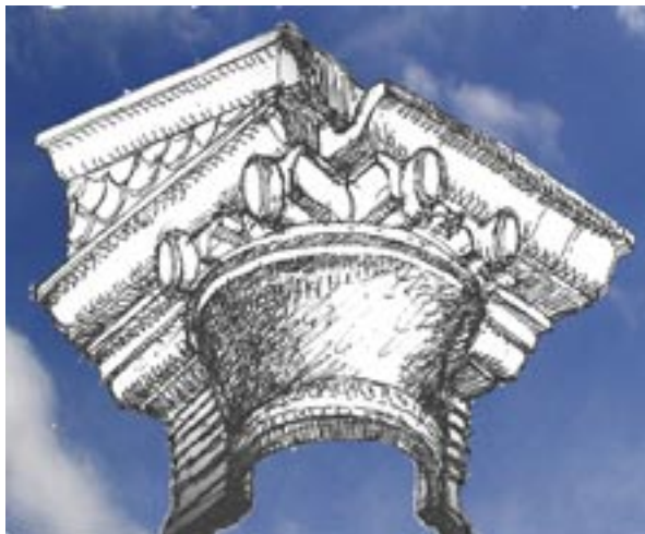
The capital to the project for Which? Headquarters in Milton Keynes was the first to be designed (in 1989) to support the 'Trabeated Raft' of a full 6th Order Entablature.
